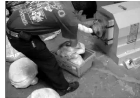
When a mold is full, detach the ingot.
