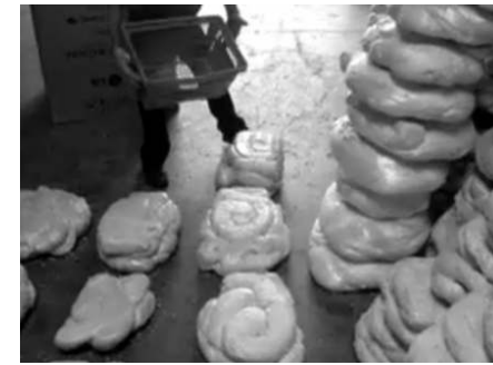
Remove the ingot from a mold. In doing so, step on the ingot to reduce the volume and give more density to it.
