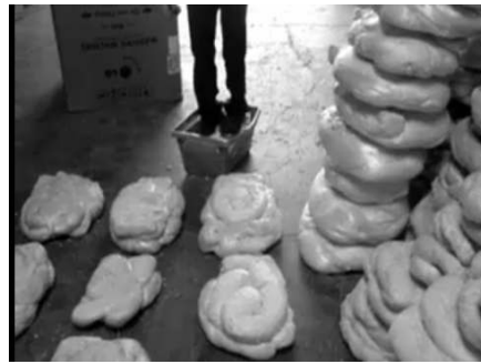
Remove the ingot from a mold. In doing so, step on the ingot to reduce the volume and give more density to it.
